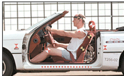
Figure 1: This is a typical pre-crash setup with the volunteer seated in an ideal position, with earphones playing loud music to create a distraction. Notice the headband he is wearing, which contains some of the sensors that record the forces associated with the crash.
