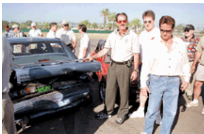
Figure 3: Aftermath of the crash illustrated in Figure 2 . This was a 36 mph closing velocity, with DV for the Lincoln and Tempo of approximately 17.5 mph.
